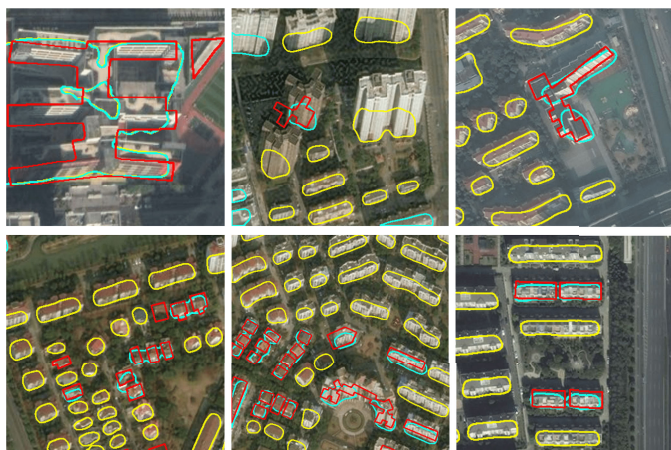
Fig. 10. Some typical failures of footprint segmentation results. The yellow, cyan, and red polygons denote the TP, FP, and FN, respectively.
