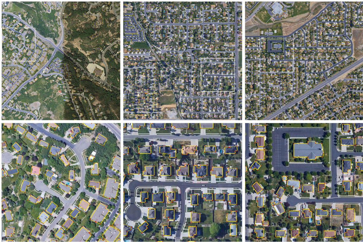
Fig. 7. Building extraction results of PolyCity in large-scale areas. PolyCity generates vector building footprints with accurate vertices, edges, and shapes even for complex scenes.
