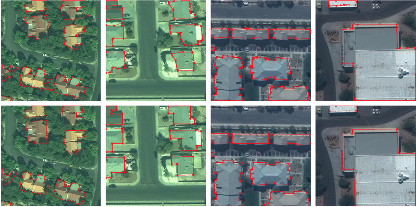
Figure 3: Qualitative comparison with state-of-the-art. The top figures show the results of ASIP (Li, Lafarge, and Marlet 2020) and the bottom figures show the results of our method. The building polygons predicted by our method have more accurate vertices in terms of locations, quantities, and angles.
