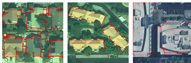
Figure 5: Three typical examples of failure cases of our proposed method. Our method fails to produce accurate polygons for buildings that are seriously sheltered by trees (left), buildings with multiple extremely short edges (middle), and high-rise buildings with serious parallax effect (right).
